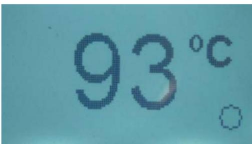
The box on the lower right of the screen is filled when heating is on –
