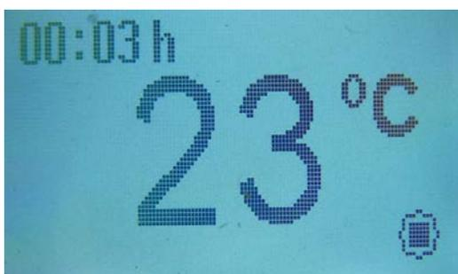
In this mode, the timer will only start once the required temperature has been reached. Note that the ‘h’ will only be visible until the timer starts.
