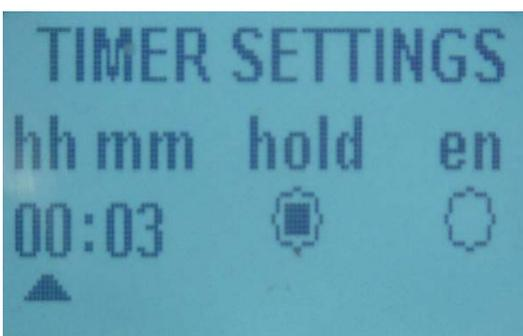
With “Hold” enabled the timer will not start until the temperature set point is reached. If “Hold” is disabled then the timer will begin as soon as the TC returns to run mode. Toggle between enabled and disabled using the  $\Delta$  or  $\nabla$  keys.
