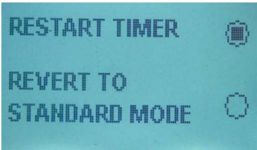
You can either select the restart option, which will start the timing cycle again with the same programmed timings, or revert to the standard mode that disables the timer and returns the controller to the normal run mode. If different timer settings are required for the next process then "Revert To Standard Mode" should be selected and the timings modified as detailed above.
